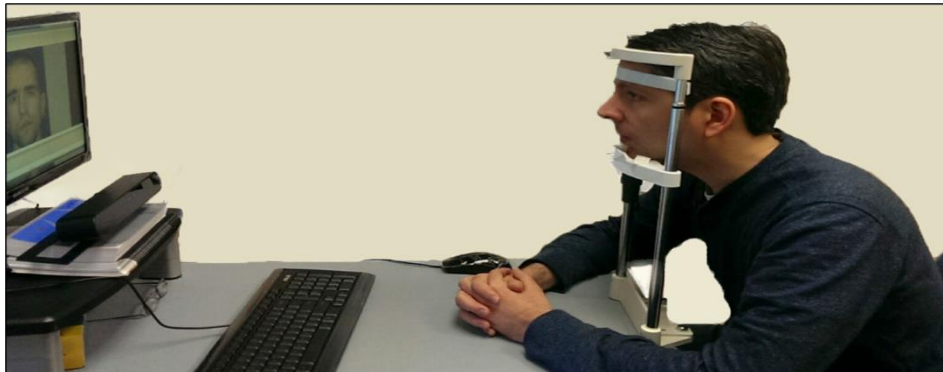
Figure 6 Our ET setup: viewing subject's face seated on a chin rest, and the near-infrared ET device aiming at the subject's eyes as he observes the monitor. The ET detects movements of less than half a degree of visual angle
